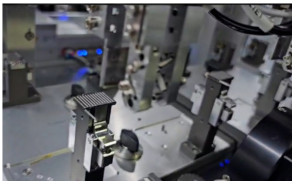
Fully Automated Busbar Insertion
